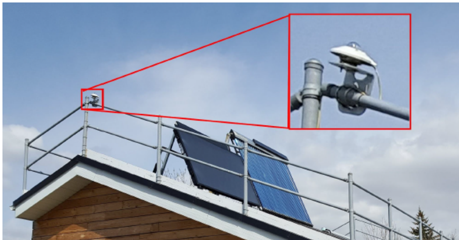
Figure 5 Solar irradiance measurement station using tilted pyranometer at SAIT Polytechnic.
